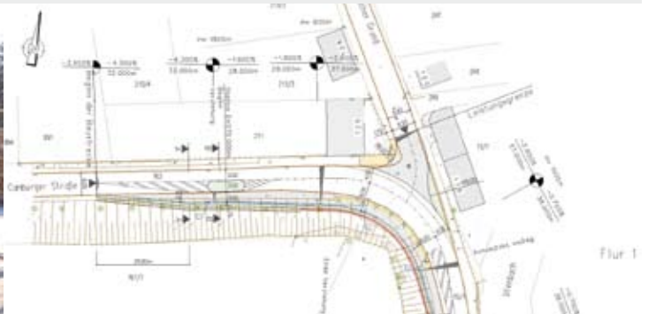
Site and elevation plan Retaining wall in the cross-town link in Utenbach
